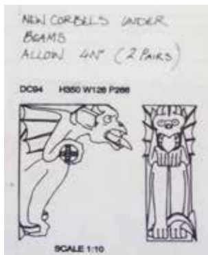
[Architectural drawing of a corbel 1996 DP]
